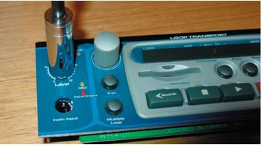
Unscrew the nut on the Headphone level pot (1/2" deep socket) and 4 hex nuts (1/4") on the back of the front panel PCB. Turn the panel face up and lift off the metal panel separating the assembly. Make sure the four white plastic standoffs remain with the metal panel. All the clear plastic actuators are loose and will fall off as soon as you tip the PCB over. Try not to touch the gold plating under the actuators, or the black contacts on the underside of the actuators themselves.
