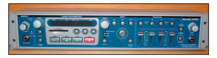
The following modification reduces output noise in the Electrix Repeater by more than 25dB, allowing the product to be used in a studio or other critical setting without adding appreciably to the noise floor. In the Repeater, the digital and analog circuitry share a common ground, and this is the source of nearly all the various noises that the machine suffers from. The modifications address this problem as well as the "tick-tick" sound that is present when playing back off the CF card.
