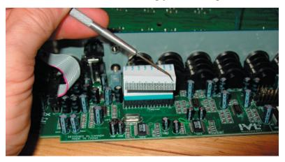
it off. This takes a bit of doing, be gentle. Be careful not to damage the plastic backing, as you need it to register the cable in the reader header.
